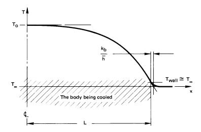
**Figure 1.11** The cooling of a body for which the Biot number,  $\overline{h}L/k_b$ , is large.
