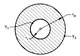
**Figure 5.25** Heat transfer through a thick, hollow sphere.
