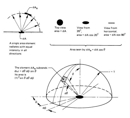
**Figure 10.4** Radiation intensity through a unit sphere.
