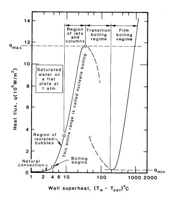
**Figure 9.2** Typical boiling curve and regimes of boiling for an unspecified heater surface.
