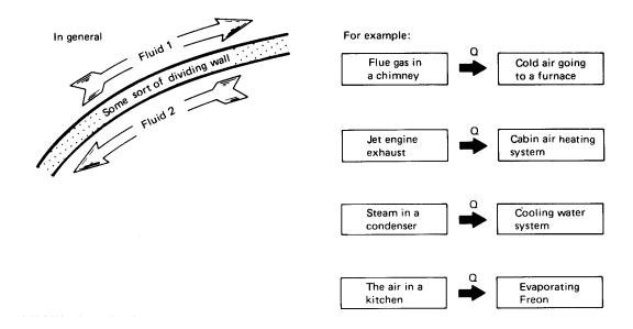
**Figure 3.1** Heat exchange.
