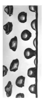
earth-normal gravity. The true width of this image is 3.48 cm. d. Film boiling of acetone on a 22 gage wire at
