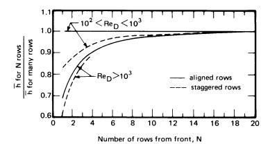
**Figure 7.15** Correction for the heat transfer coefficients in the front rows of a tube bundle [7.28].
