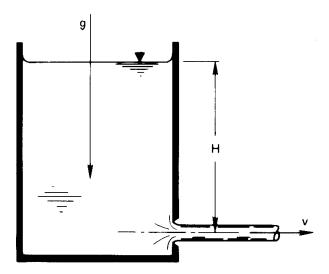
**Figure 4.4** Efflux of liquid from a tank.
