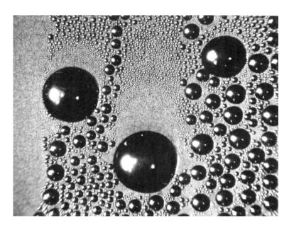
**b.** Typical photograph of dropwise condensation provided by Professor Borivoje B. Mikić. Notice the dry paths on the left and in the wake of the middle droplet.
