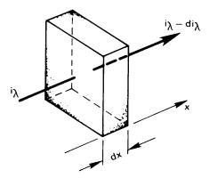
**Figure 10.20** The attenuation of radiation through an absorbing (and/or scattering) gas.
