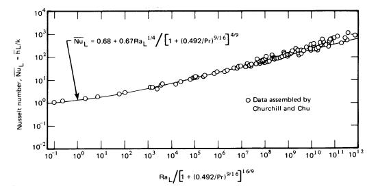
**Figure 8.3** The correlation of  $\overline{h}$  data for vertical isothermal surfaces by Churchill and Chu [8.3], using Nu<sub>L</sub> = fn(Ra<sub>L</sub>, Pr). (Applies to full range of Pr.)
