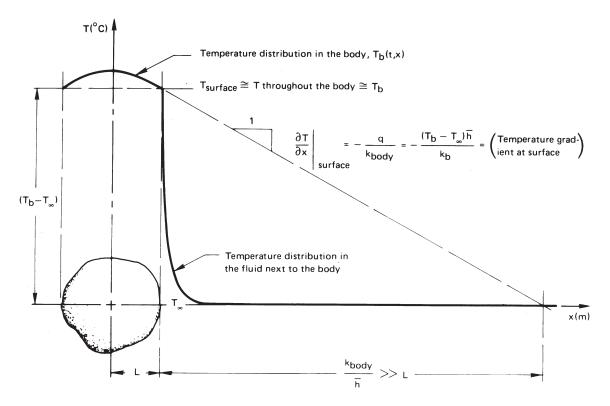
**Figure 1.10** The cooling of a body for which the Biot number,  $\overline{h}L/k_b$ , is small.
