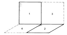
**Figure 10.12** Radiation between two offset perpendicular squares.
