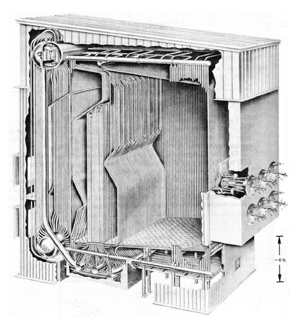
**Figure 3.12** The heat exchange surface for a steam generator. This PFT-type integral-furnace boiler, with a surface area of  $4560~\text{m}^2$ , is not particularly large. About 88% of the area is in the furnace tubing and 12% is in the boiler (Photograph courtesy of Babcock and Wilcox Co.)
