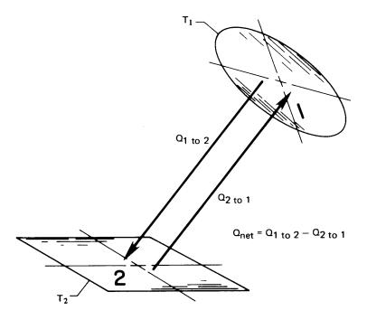
Figure 10.1 Thermal radiation between two arbitrary surfaces.
