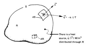
**Figure 2.4** Control volume in a heat-flow field.
