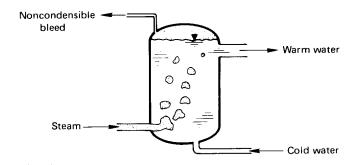
Figure 3.2 A direct-contact heat exchanger.
