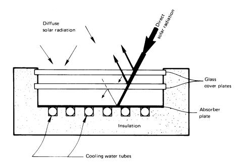
Figure 10.26 A typical flat-plate solar collector.
