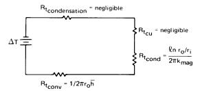
**Figure 2.15** Thermal circuit for an insulated tube.
