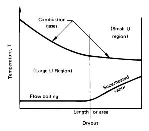
**Figure 3.11** A typical case of a heat exchanger in which U varies dramatically.
