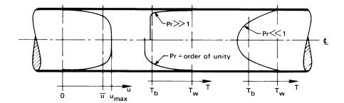
**Figure 7.7** Velocity and temperature profiles during fully developed turbulent flow in a pipe.
