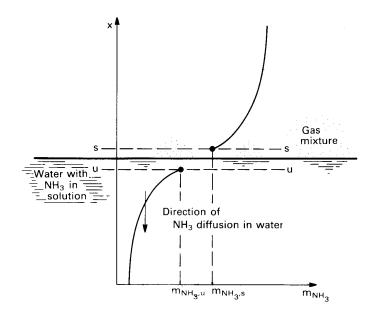
Figure 11.9 Absorption of ammonia into water.
