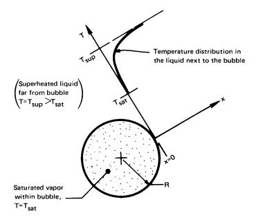
**Figure 5.17** A bubble growing in a superheated liquid.
