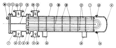
c) Two tube-pass, two shell-pass exchanger
