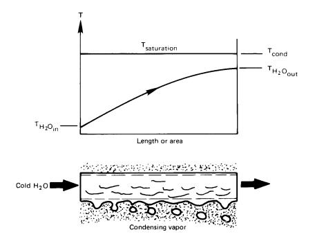
**Figure 3.9** The temperature distribution through a condenser.
