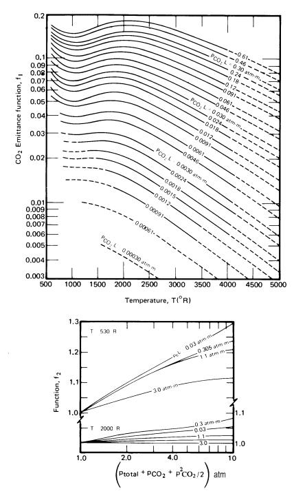
**Figure 10.23** Functions used to predict  $\varepsilon_g=f_1f_2$  for CO<sub>2</sub> in air. All pressures in atmospheres.
