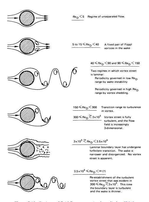
Figure 7.10 Regimes of fluid flow across circular cylinders [7.24].
