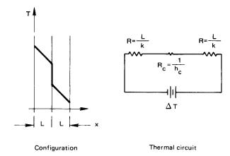
**Figure 2.11** Conduction through two unit-area slabs with a contact resistance.
