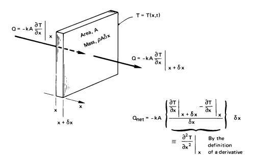
**Figure 1.8** One-dimensional heat conduction through a differential element.
