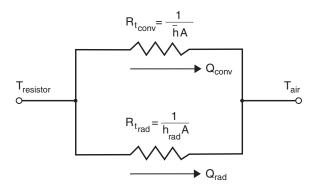
**Figure 2.17** An electrical resistor cooled by convection and radiation.
