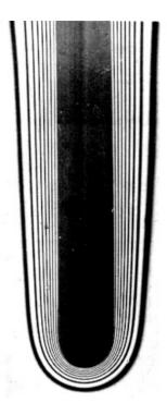
**a.** A 1.34 cm wide flat plate with a rounded leading edge in air.  $T_w = 46.5$  °C,  $\Delta T = 17.0$  °C,  $Gr_{radius} \simeq 2250$
