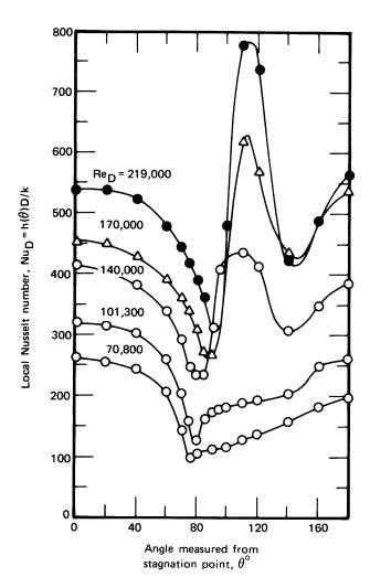
**Figure 7.12** Giedt's local measurements of heat transfer around a cylinder in a normal cross flow of air.
