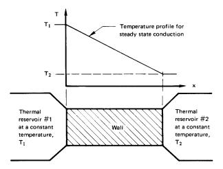
**Figure 1.2** Irreversible heat flow between two thermal reservoirs through an intervening wall.
