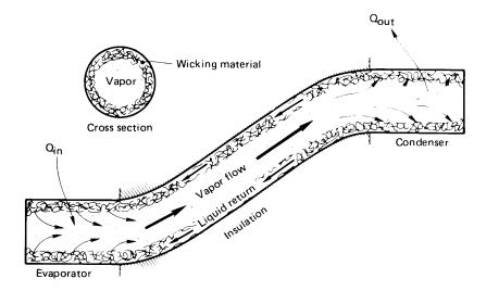
**Figure 9.22** A typical heat pipe configuration.
