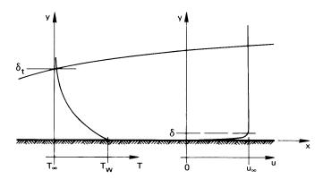
**Figure 6.15** A laminar b.l. in a low-Pr liquid. The velocity b.l. is so thin that  $u \simeq u_{\infty}$  in the thermal b.l.
