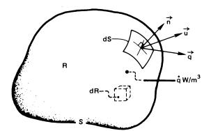
**Figure 6.12** Control volume in a heat-flow and fluid-flow field.
