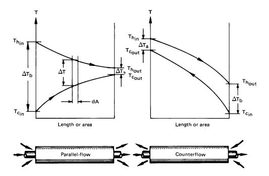
**Figure 3.8** The temperature variation through single-pass heat exchangers.
