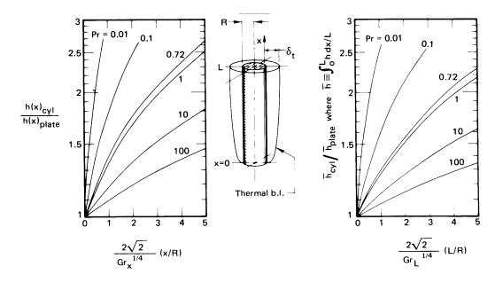
**Figure 8.7** Corrections for h and  $\overline{h}$  on vertical isothermal plates to make them apply to vertical isothermal cylinders [8.11].
