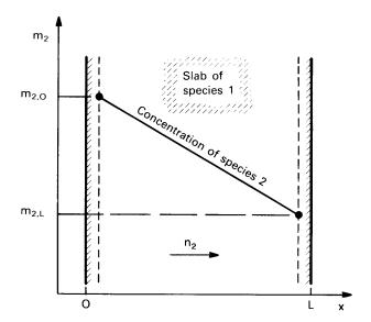
**Figure 11.12** One-dimensional, steady diffusion in a slab.
