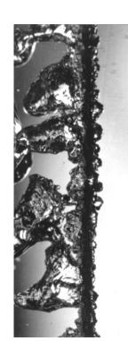
3.75 cm length of 0.164 cm diam. wire in benzene at earth-normal gravity.  $q=0.35\times10^6~\mathrm{W/m^2}$
