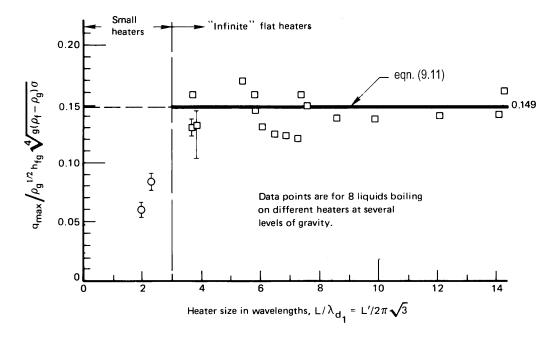
**Figure 9.12** Comparison of the  $q_{\text{max}}$  prediction for infinite horizontal heaters with data reported in [9.18].
