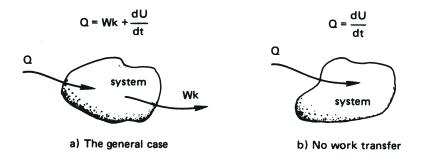
**Figure 1.1** The First Law of Thermodynamics for a closed system.
