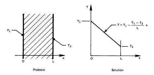
**Figure 2.7** Heat conduction in a slab (Example 2.2).
