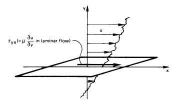
**Figure 6.18** The shear stress,  $\tau_{\gamma x}$ , in a laminar or turbulent flow.
