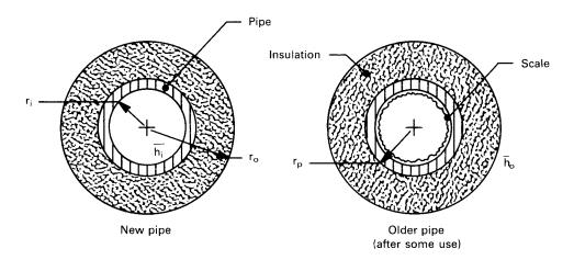
**Figure 2.21** The fouling of a pipe.
