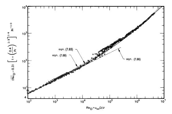
**Figure 7.13** Comparison of Churchill and Bernstein's correlation with data by many workers from several countries for heat transfer during cross flow over a cylinder. (See [7.26] for data sources.) Fluids include air, water, and sodium, with both  $q_w$  and  $T_w$  constant.
