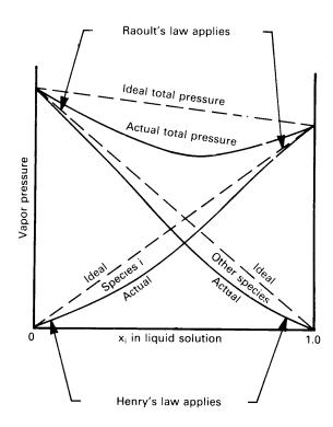
**Figure 11.10** Typical partial and total vapor-pressure plot for the vapor in contact with a liquid solution, illustrating the regions of validity of Raoult's and Henry's laws.
