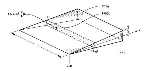
Figure 4.12 A two-dimensional wedge-shaped fin.
