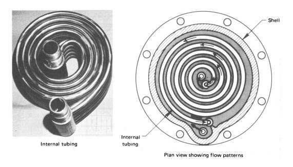
**Figure 3.4** Heliflow compact counterflow heat exchanger. (Photograph coutesy of Graham Manufacturing Co., Inc., Batavia, New York.)
