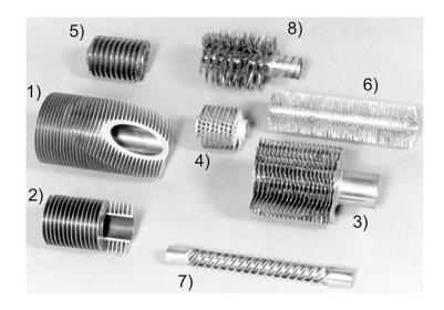
**a.** Eight examples of externally finned tubing: 1) and 2) typical commercial circular fins of constant thickness; 3) and 4) serrated circular fins and dimpled spirally-wound circular fins, both intended to improve convection; 5) spirally-wound copper coils outside and inside; 6) and 8) bristle fins, spirally wound and machined from base metal; 7) a spirally indented tube to improve convection and increase surface area.
