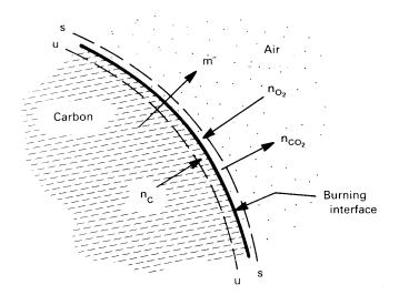
**Figure 11.4** Low-temperature carbon oxidation.
