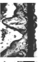
b. Two views of transitional boiling in acetone on a 0.32 cm
