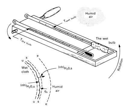
**Figure 11.20** The wet bulb of a sling psychrometer.
