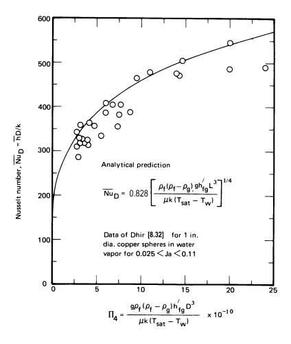
**Figure 8.10** Correlation of the data of Dhir [8.32] for laminar film condensation on spheres at one value of Pr and for a range of  $\Pi_4$  and Ja, with properties evaluated at  $(T_{\text{sat}} + T_w)/2$ . Analytical prediction from [8.33].
