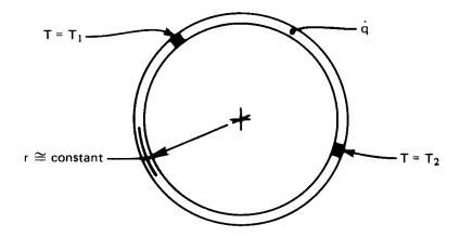
**Figure 4.2** One-dimensional heat conduction in a ring.
