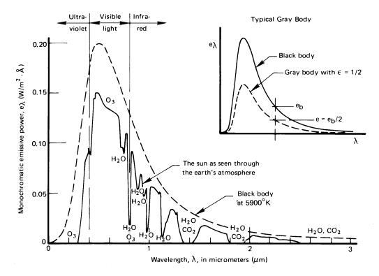
**Figure 10.2** Comparison of the sun's energy as typically seen through the earth's atmosphere with that of a black body having the same mean temperature, size, and distance from the earth. (Notice that  $e_{\lambda}$ , just outside the earth's atmosphere, is far less than on the surface of the sun because the radiation has spread out over a much greater area.)
