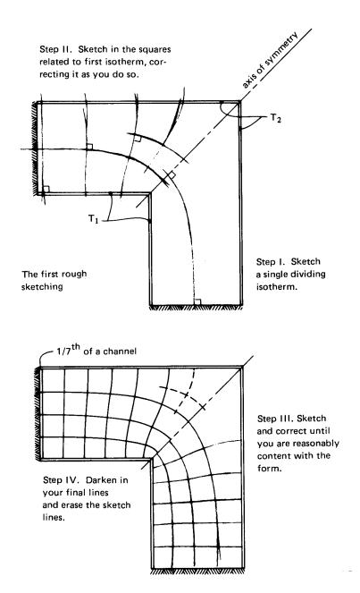
**Figure 5.21** The evolution of a flux plot.
