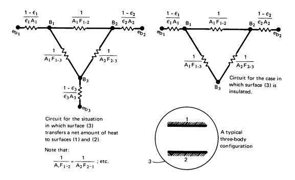
**Figure 10.15** The electrical circuit analogy for radiation among three gray surfaces.
