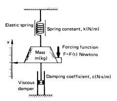
**Figure 5.2** A spring-mass-damper system with a forcing function.
