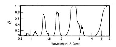
**Figure 10.21** The monochromatic absorptance of a 1.09 m thick layer of steam at  $127^{\circ}\text{C}$ .
