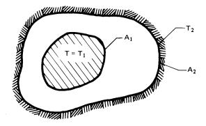
**Figure 10.14** Heat transfer between an enclosed body and the body surrounding it.
