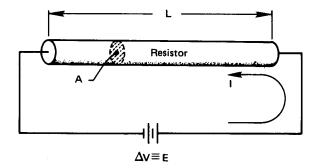
**Figure 2.9** The one-dimensional flow of current.
