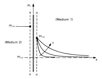
**Figure 11.13** Mass diffusion into a semi-infinite stationary medium.
