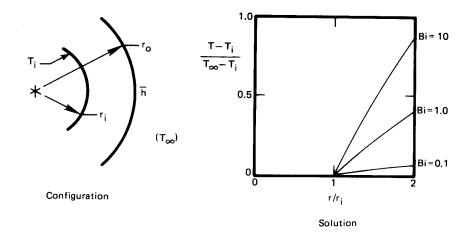
**Figure 2.13** Heat transfer through a cylinder with a convective boundary condition (Example 2.6).
