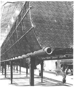
Above and left: A very large feed-water preheater. Tubes are shown withdrawn from the shell on the left. Inset above shows baffles before tubes are inserted. (Photos courtesy of Southwest Engineering Co., Subsidiary of Cronus Industries, Inc., Los Angeles, Calif.)
