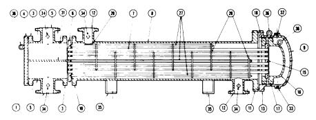
b) One shell-pass, two tube-pass exchanger
