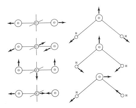
Figure 10.19 Vibrational modes of carbon dioxide and water.
