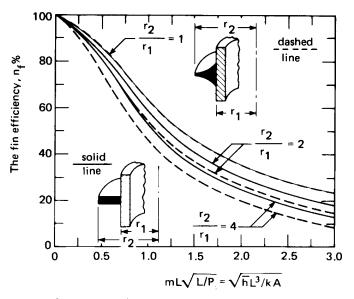
Comparison of a constant thickness circular fin, and a hyperbolic fin with thickness inversely proportional to radius. (L  $\equiv$  r<sub>2</sub> - r<sub>1</sub> and m is based on the area, A, shown in black.)
