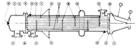
a) Single shell-pass, single tube-pass exchanger
