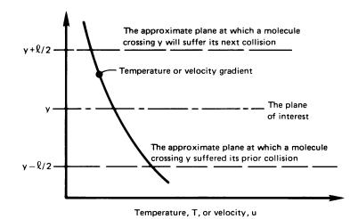
**Figure 6.13** Momentum and energy transfer in a gas with a velocity or temperature gradient.
