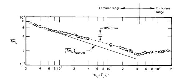
**Figure 8.15** Film condensation on vertical plates. Data are for water [8.40].
