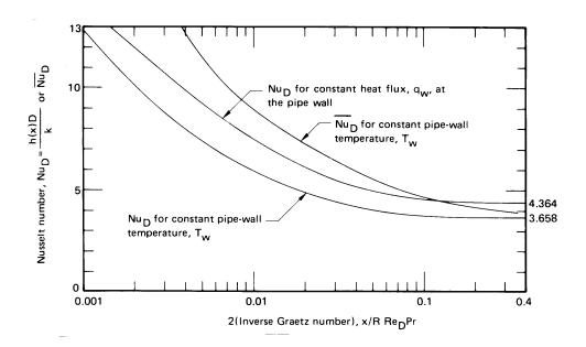
**Figure 7.4** Local and average Nusselt numbers for the thermal entry region in a hydrodynamically developed laminar pipe flow.
