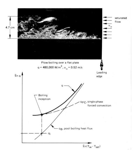
Figure 9.17 Forced convection boiling on an external surface.
