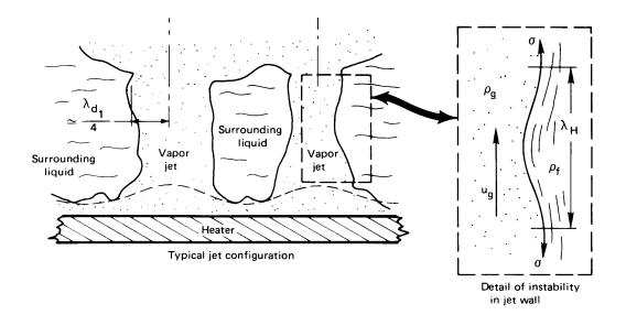
Figure 9.11 Helmholtz instability of vapor jets.
