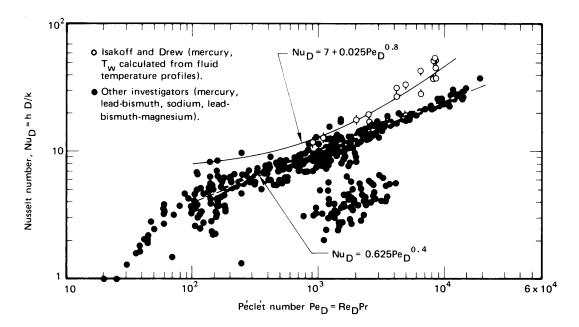
**Figure 7.8** Comparison of measured and predicted Nusselt numbers for liquid metals heated in long tubes with uniform wall heat flux,  $q_w$ . (See NACA TN 336, 1955, for details and data source references.)
