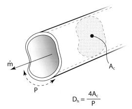
**Figure 7.9** Flow in a noncircular duct.
